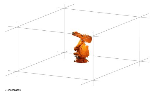
Absolute Accuracy is a TCP calibration in order to reach a good positioning in the Cartesian coordinate system.
